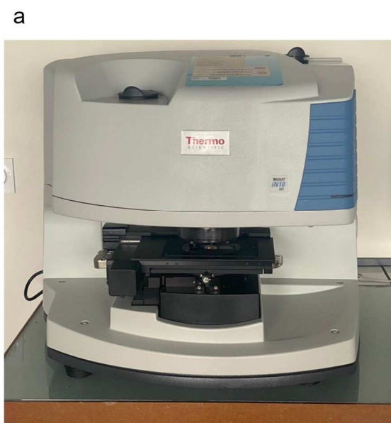
FIGURE 18A – PHOTOGRAPH OF THE NICOLET iN10 USED FOR MICROPLASTIC ANALYSIS; B – PHOTOGRAPH OF THE NICOLET iS5 USED FOR THE CHARACTERIZATION OF MACROLITTER.
